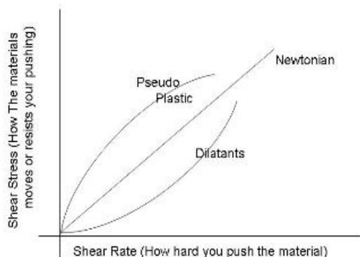
Figure 2: Newtonian and non-Newtonian fluids
