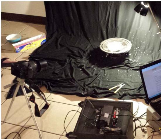
Figure 4: Experimental setup, including camera, speaker, amplifier, laptop, and lighting (black light bulb used when original image was taken)
