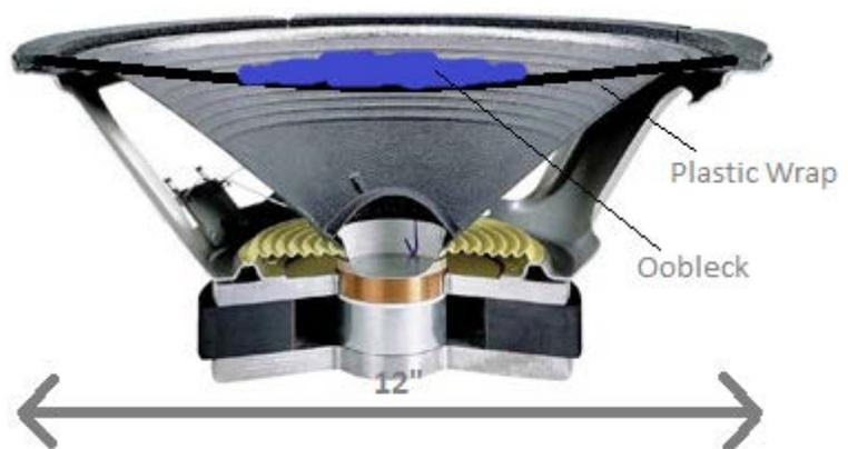
Figure 1: Experimental setup of the speaker
